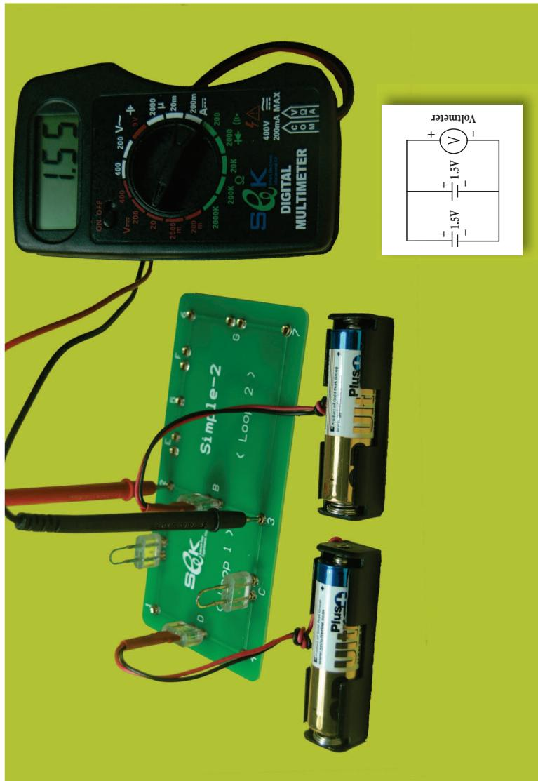
4. Insert the red probe of the DMM in the point (2) & black probe in the point (3), watch the DMM reading.
