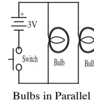
8. Insert a switch at the pair (I), bulb 3.8V at the pair (K), another bulb 3.8V at the pair (N) and jumpers at the pairs (A, H, M, L) as shown in the above diagram.
