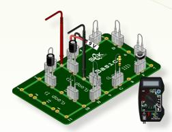
Power Supply Board (PSB): (Voltage Source): There are six AA type 1.5V batteries present in the board. There are also seven outlets that can be adjusted to multiple DC output voltages (1.5, 3, 4.5, 6 and 7.5 volts). The outlets can be connected to the Basics Board and other experiment boards with the use of a connection wire.
